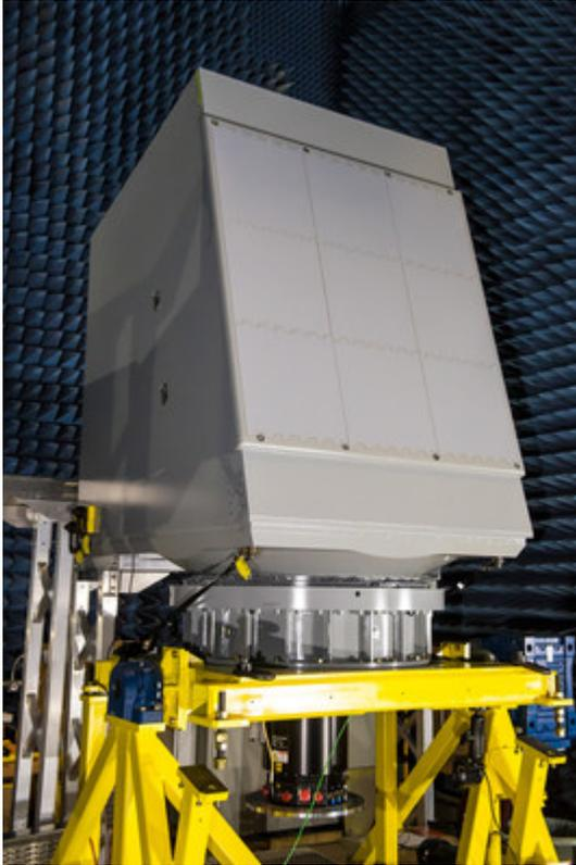
EASR is the Navy's next generation radar for aircraft carriers and amphibious warfare ships that provides simultaneous anti-air and anti-surface warfare, electronic protection and air traffic control capabilities.
