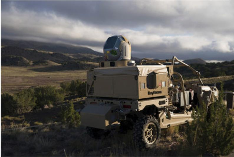
The HEL system, paired with Raytheon's Multi-spectral Targeting System, uses invisible beams of light to defeat hostile UASs. Mounted on a Polaris MRZR all-terrain vehicle, the system detects, identifies, tracks and engages drones.
